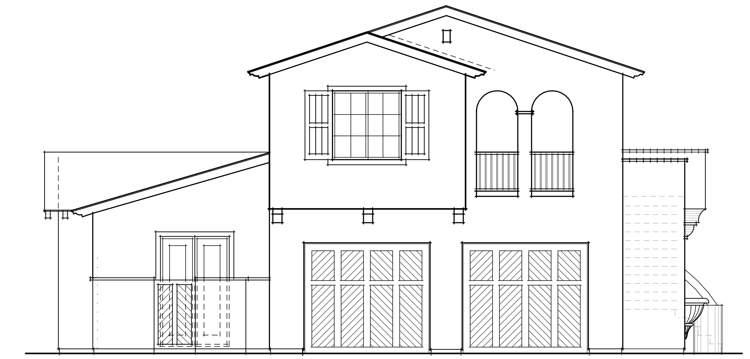
CASITA/ CARRIAGE UNIT FRONT ELEV 'A'
